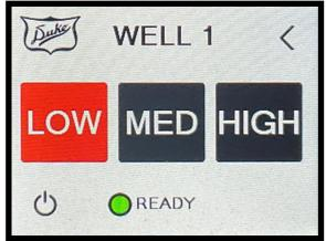
On a multi-well unit, press the ON/OFF icon to turn ON/OFF an individual well.
