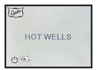
3 The main runtime screen will appear. If the unit contains more than one well, the screen will show an icon for each well. On a multi-well unit, press an icon for a well to turn on.
