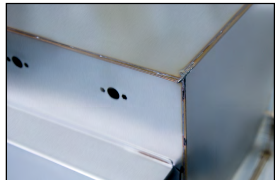
Fully laser-welded oven cavity
