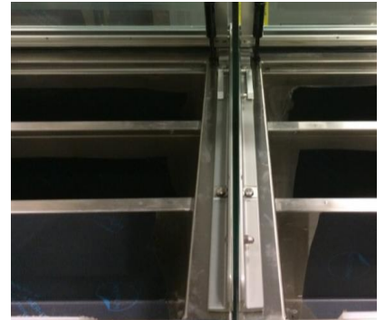
End glass must be bolted tight between the end mounts, without gaps. If gaps are present, ensure the hex bolts are loosened on all units.
