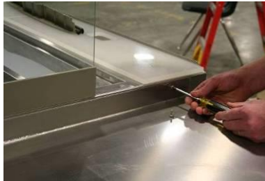
Install screws through the upturned flange of the cashier to the cold pan.
