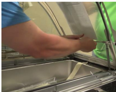
Using Philips screw driver, install the bolts that come with hot food units into the two arms on left and right side.
