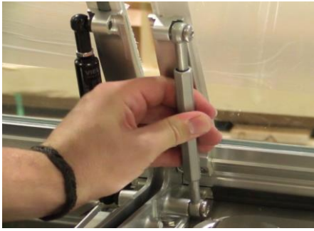
To adjust the hot food front glass, turn the middle section of connecting rod.
