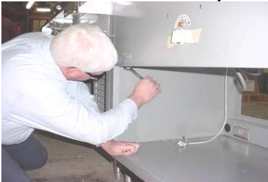
Bolt cold pan unit to hot food and cashier unit to cold pan.
