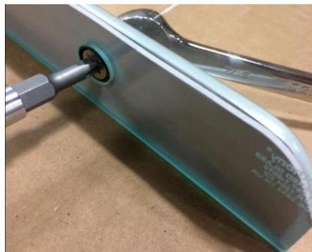
Use provided 1/4-20 Flat Head Screw to make it flush with glass and avoid interference.
