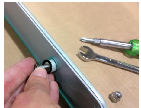
Don't forget to include the black plastic washer and the white plastic spacer for glass.
