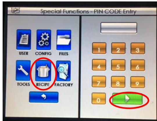
2. Press the Recipe button, enter the pin code "5678", then press the button
